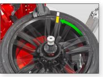
The bead rollers safely hold the tire stationary while the rim is rotated to complete match-mounting.
